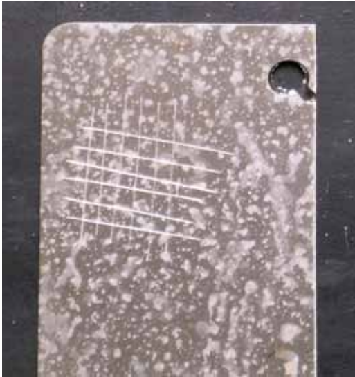
Panel cleaned with VpCI-429 and then coated with VpCI-386 Clear
